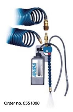
The ARIANA Micro System for minimum quantity lubrication uses a coaxial spray nozzle to produce a round spray with spraying angle. It is possible to produce different spray cones for many application areas by rotating the cap. The coaxial spray nozzle is operated pneumatically and is supplied with the medium by means of a separate, unpressurized tank.
